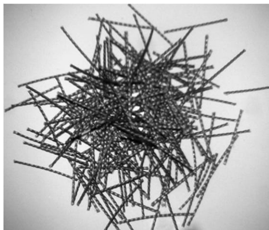
Fig. 2. Tire cord with 20 mm length.
